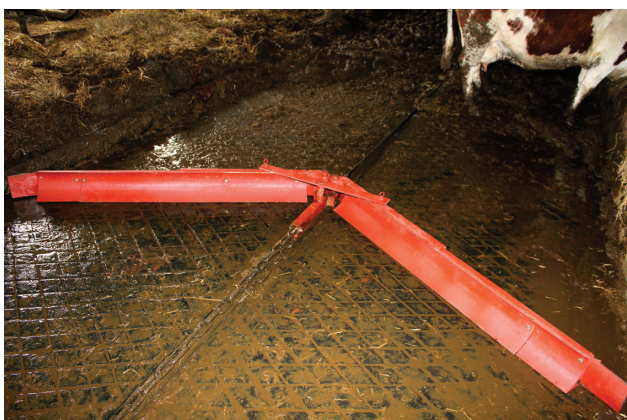
Fig. 1. Scraper unit with scrapers in the form of a blade
