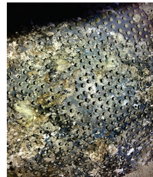
Fig. 10. Solid glassy deposits on the grate surface when the gasifier operated at an 80 % straw content in the fuel
