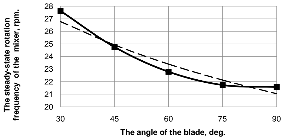
Fig. 6 - The graphical dependence of the mixer steady-state rotation frequency on the angle of the blades ..... - theoretical values; - experimental values
